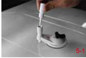
6. Set the pressure drive into the injection tube and pressure the resin into the crack area.
