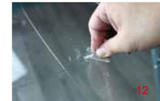
12. Move the car into direct sunlight or use UV light for 5-10 minutes with cure process. <don't remove the curing strip at this point>
