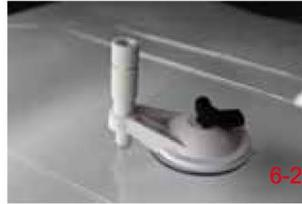
7. Allow approximately 4-6 minutes for the repair resin to be absorbed into the damage area.
